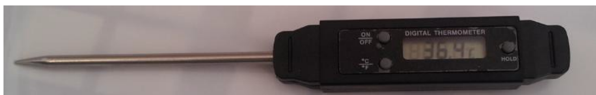
Figure 3 - Example of an approved temperature measuring device accurate to \pm 1^{\circ}\text{C}
