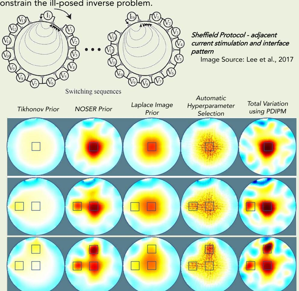
Image processing using ImageJ revealed that for 1 hole damage, Laplace Image Prior gave a normalised area and perimeter closest to the damage. Although NOSER and Total Variation using PDIPM identified the location of all three defects, the size and shape were not represented accurately.
